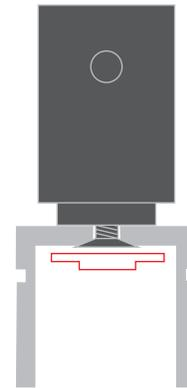
5. Insert the rod into the mounting bracket of the head. Block the rod by tightening the pressure screw in the head with the Allen wrench.
